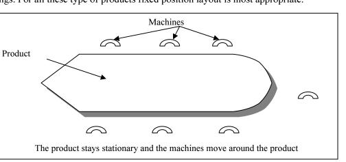
Figure 10.1.3: Typical fixed position Layout
