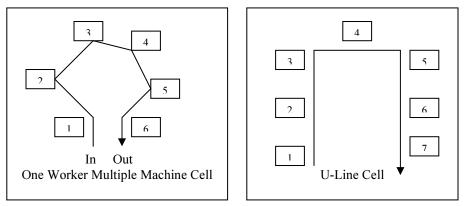
Figure 10.4.1: Example of OWMM and U-Line cell
