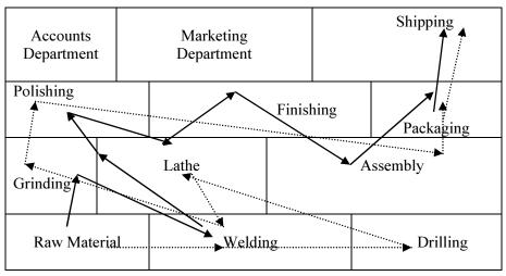
Figure 10.1.1: Typical process layout format
