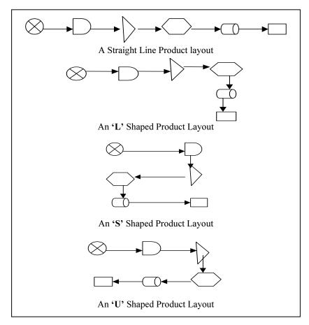
Figure 10.1.2: Typical process layout formats
