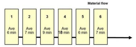
In the diagram above, the material is flowing from left to right and passes through six process steps. Process step four is by far the longest and takes twice as long as step three. Assuming all process steps keep working, it will not take long for a queue to form in front of process step four. Process step four is the bottleneck. It does not matter how fast or how long the other process steps operate because the output of the total process is determined by the performance at process step four.
