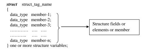
Here, the *struct\_tag\_name* is called structure tag name and it is optional and each member definition is a normal variable definition, such as *int a, float b, char c or char c[]* etc; or any other valid variable
