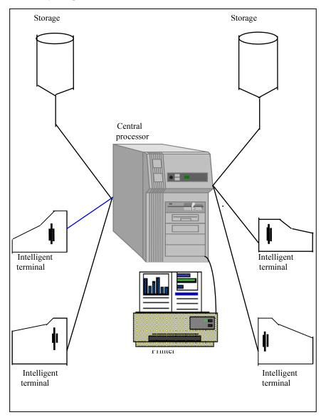
Fig. 2.5: Distributed-logic system.
