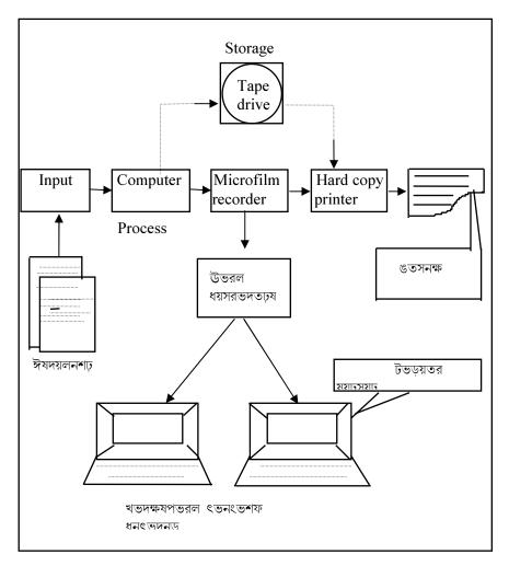
Fig. 2.8 : A schematic diagram of COM production system.
